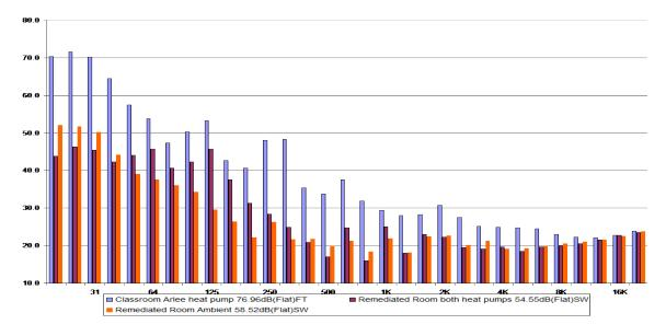
064 Hz Reduced from 53 dB to 42 dB. 125 Hz Reduced from 52 dB to 33 dB. 250 Hz Reduced from 48 dB to 28 dB. 500 Hz Reduced from 30 dB to 20 dB. 1 K Hz Reduced from 30 dB to 20 dB.
