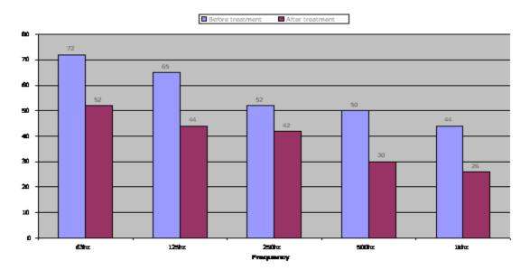
The above graph shows decibel reduction on two large units with only 3/8" LP-13 Shake Absorber<sup>®</sup> material used on top of a roof curb.
